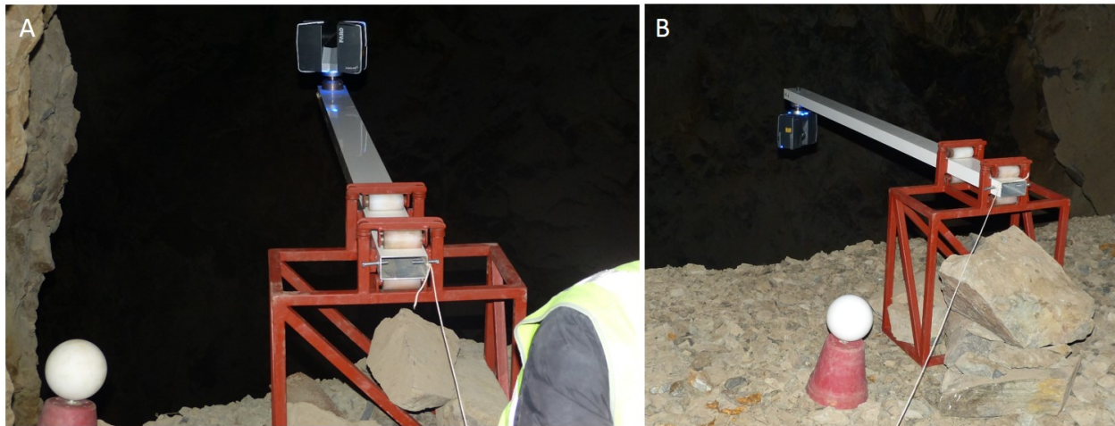
Figure 48: 3D laser scanner (Faro Focus3D S120) with support scanning the 2075E stope
