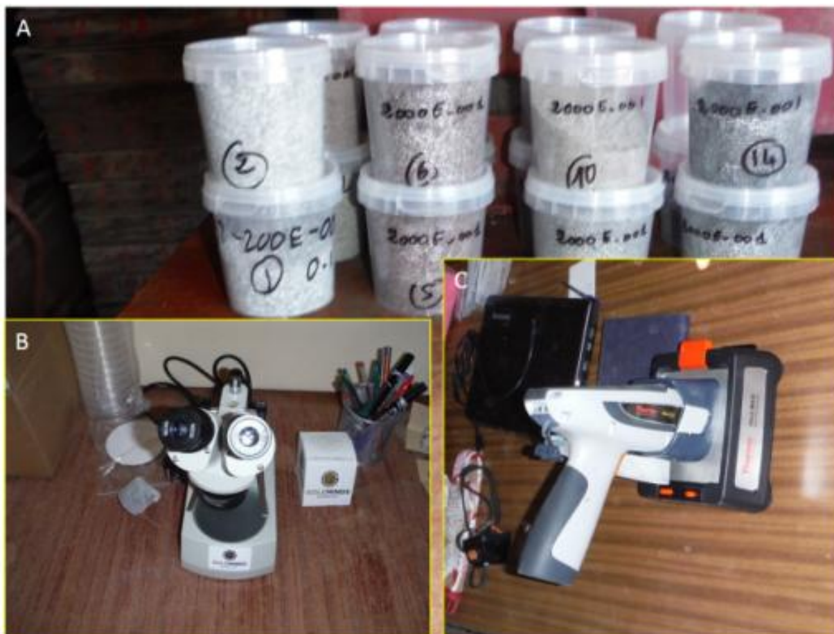
Figure 64: A) Composite samples taken after the drying process. B) Binocular microscopy used for petrographic analyses of select samples. C) Niton XL3t XRF used to analyze small samples (~ 5g)
