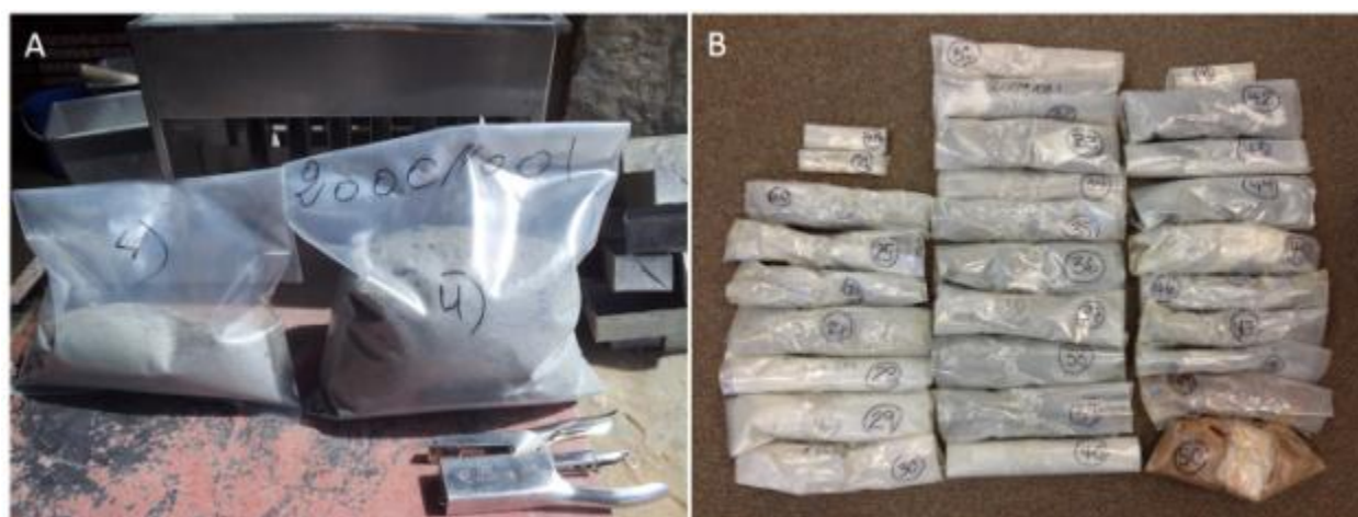
Figure 65: A) YAK sample (cuttings); the plastic bag on the left corresponds to a quarter of the cuttings prepared to be sent to ALS laboratory, the other plastic bag is kept in the core shack for archives. B) Percussion drill samples taken by the T28 drill hammer
