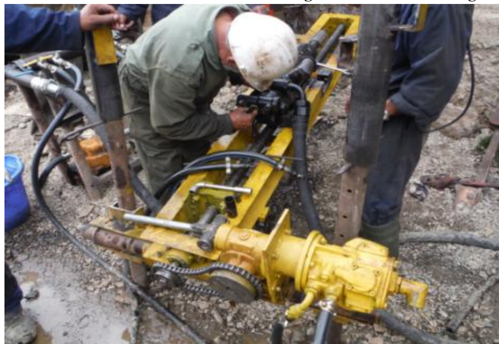
Figure 57: YAK percussion drill on a steel frame at the entrance of the 2000 level
