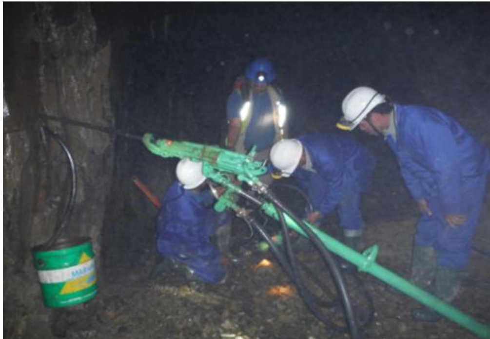
Figure 56: T28 drill in eastern zone of 2000 level. The green bucket is collecting the cuttings
