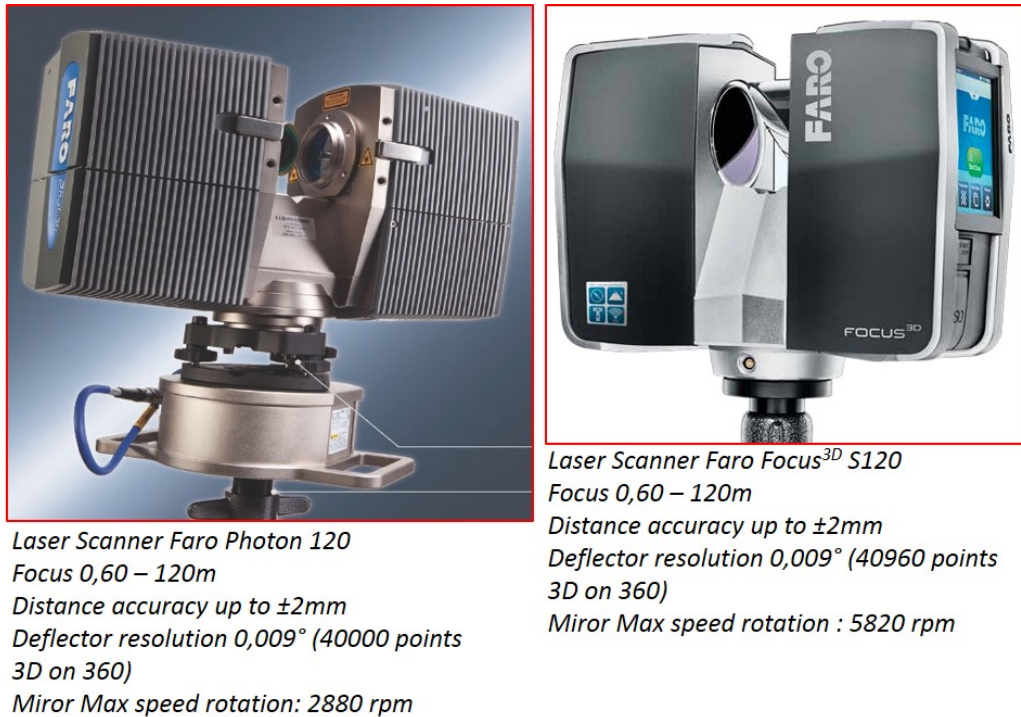
Figure 46: The laser scanner used for the underground 3D monitoring survey
