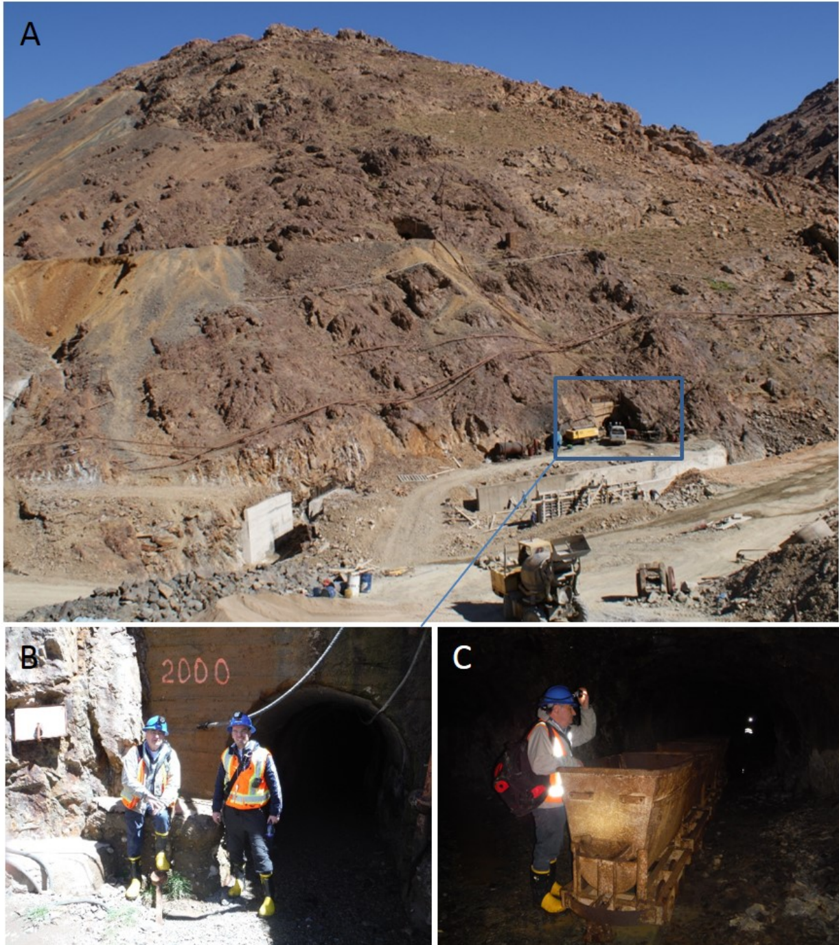
Figure 21: A) A view looking east showing the entrance of the 2000 and 2025 adits, a network of water pipes and several bridges were in construction at the time of this photo. B) The entrance of the 2000 level before recent modifications. C) An old small mine car on railway at the 2000 level.
