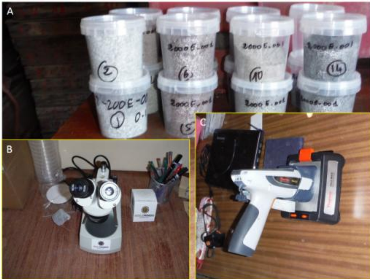
Figure 64: A) Composite samples taken after the drying process. B) Binocular microscopy used for petrographic analyses of select samples. C) Niton XL3t XRF used to analyze small samples (~ 5g).
