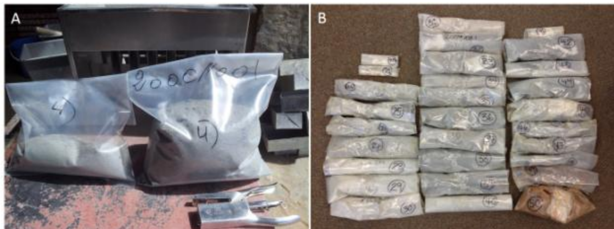
Figure 65: A) YAK sample (cuttings); the plastic bag on the left corresponds to a quarter of the cuttings prepared to be sent to ALS laboratory, the other plastic bag is kept in the core shack for archives. B) Percussion drill samples taken by the T28 drill hammer.
